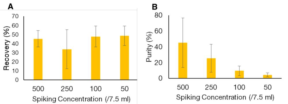
**Recovery and purity of spiked cells after ClearCell® FX enrichment.** Varying concentrations of NCI-H1975 were spiked into 7.5 ml of blood and processed on ClearCell® FX. (A) Recovery of NCI-H1975 cells was on average 44.5% (s.d. 14.2%). (B) Purity of spiked cells recovered ranged between 0.7% and 83.2%, depending on the number of cells spiked and the number of leukocytes in the output.
